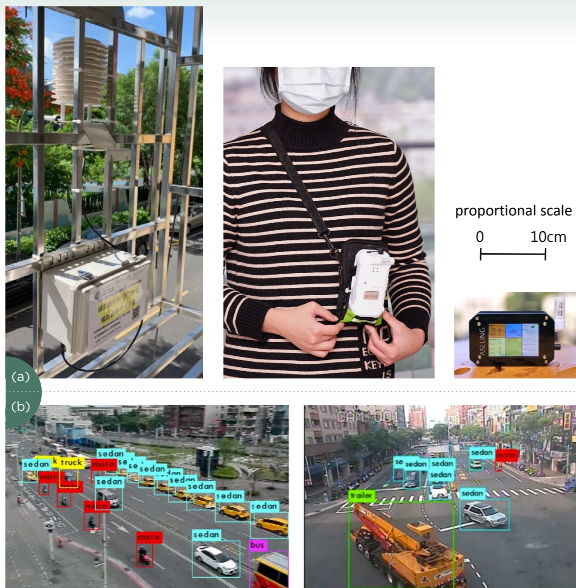
Figure 2. Scientific tools developed in this study including (a) outdoor (AS-LUNG-O, left), portable (AS-LUNG-P, middle), and indoor (AS-LUNG-I, right) PM_{2.5} micro-sensors, and (b) a traffic analysis system that classifies/counts vehicles in five categories (motorcycle in red, sedan in blue, bus in purple, truck in yellow, and trailer in green).
